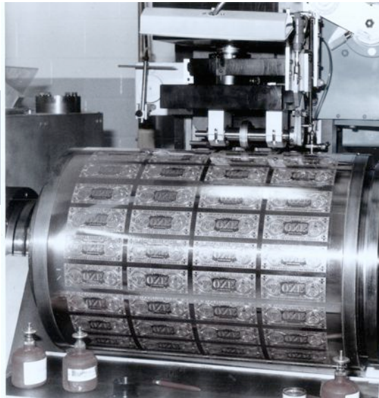
BEP's Web Currency Press plate cylinder with engraved $1 FRN's - this plate weighed close to 1 ton. It was heavy and very large with 96 images or currency notes engraved around the plate.
